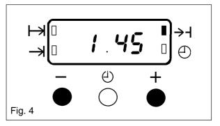
The 'Countdown' will sound intermittently for up to 2 minutes at the end of the timed period. The sound can be stopped by pressing any button.
